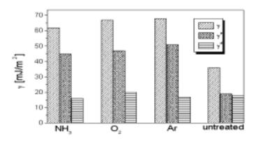
FIGURE1. Comparison of surface free energy and its components before and after the treatment in Ar, NH<sub>3</sub> and O<sub>2</sub> discharges. The domain represents the types of the sample. The treatment conditions were P = 100W, Q = 52 sccm, p= 36.5 Pa, and exposure time t = 10 min. The bias voltages U<sub>bias</sub> were -20, -25, -30 V for ammonia, oxygen and argon discharges respectively.
