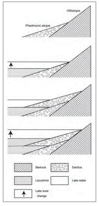
**Figure 8**. Schematic diagram showing development of interfinger of piedmont slope deposits and lacustrine sediments as lake level rose (chronologically, from top to bottom)
