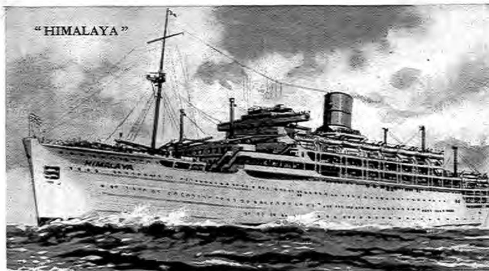
R.M.S. "Himalaya."—Peninsula and Oriental Steam Navigation Co. Built 1948 by Vickers Armstrong, Ltd. Weight, 29,000 tons; Service speed, 22 knots; Length, 710 ft.; Breadth, 90 ft. Passengers, 779 First Class, 393 Tourist Class. Cargo capacity, 6,000 tons. Twin-screw turbines developing 42,500 h.p.
