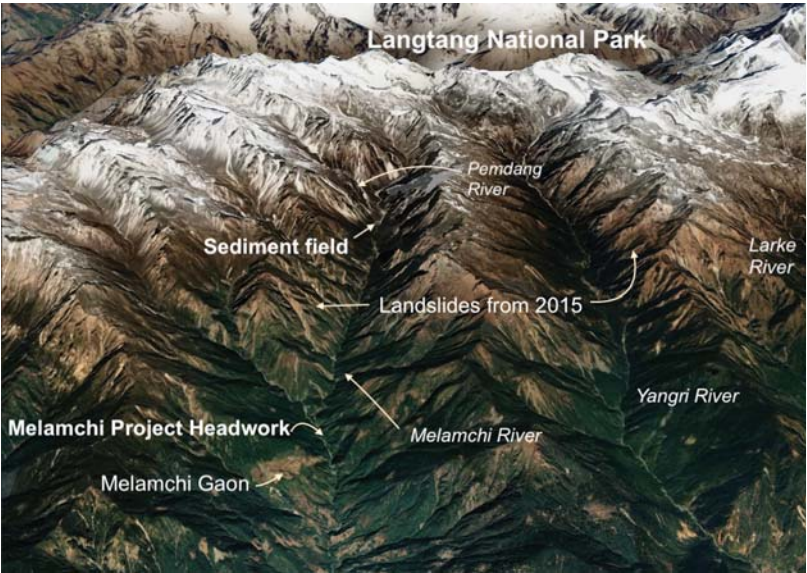
The 26.5 km tunnel that brought 170 million litres of water daily from Melamchi to Kathmandu for 3 months before its headwork was damaged by the floods on 15 and 30 July 2021 (above). Google Earth image of the Melamchi Valley taken in December 2017 (below) showing landslide scars and the location of the sediment field near the confluence of the Melamchi and Pemdang rivers.
