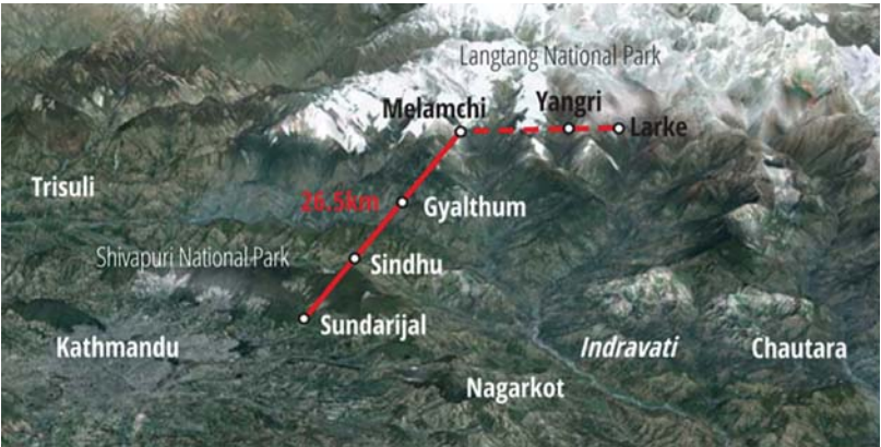
The 26.5 km tunnel that brought 170 million litres of water daily from Melamchi to Kathmandu for 3 months before its headwork was damaged by the floods on 15 and 30 July 2021 (above). Google Earth image of the Melamchi Valley taken in December 2017 (below) showing landslide scars and the location of the sediment field near the confluence of the Melamchi and Pemdang rivers.
