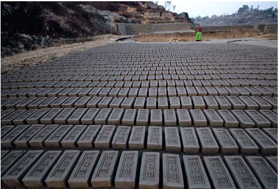
Bricks are laid out to dry after being cast. A single kiln can produce up to 70, 000 bricks a day. Each brick is sold for Rs 3.5.
