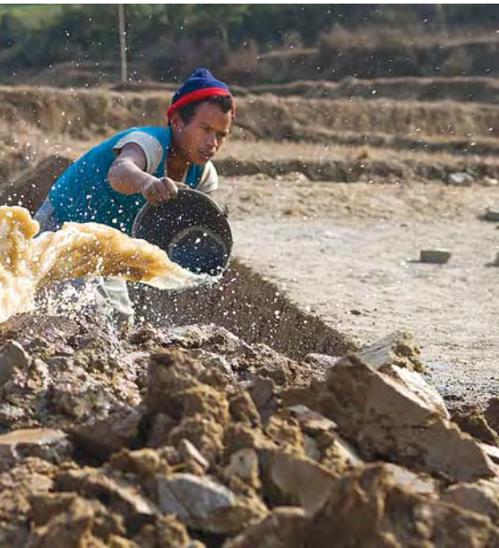
A worker wets soil with water drained from nearby streams to form mud for moulding bricks.
